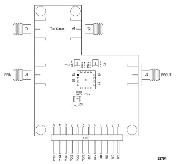
Figure 3. SKY65375-11 Evaluation Board Assembly Diagram
