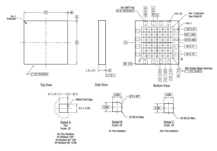
Dimensioning and tolerancing according to ASME Y14.5M-1994. All measurements are in millimeters
