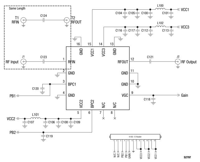
Figure 6. SKY65375-11 Evaluation Board Schematic
